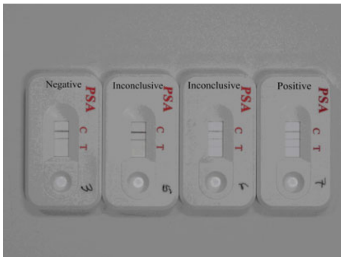
FIG. 9—Photograph illustrating various results obtained from the analysis of serial dilutions of a minimal PSA standard solution. No test line can be seen in the membrane at far left (Terminated Program PSA concentration <0.35 ng/mL) and this result would be recorded as “negative.” Slightly more concentrated solutions result in very weak test lines that have Terminated Program results between 0.35 and 0.55 ng PSA/mL (middle two membranes). These results would be recorded as “inconclusive.” At far right, a slightly more concentrated solution (Terminated Program PSA result >0.55 ng/mL) results in a visible test line that is strong enough to be recorded easily by photography which would be recorded as “positive.”
