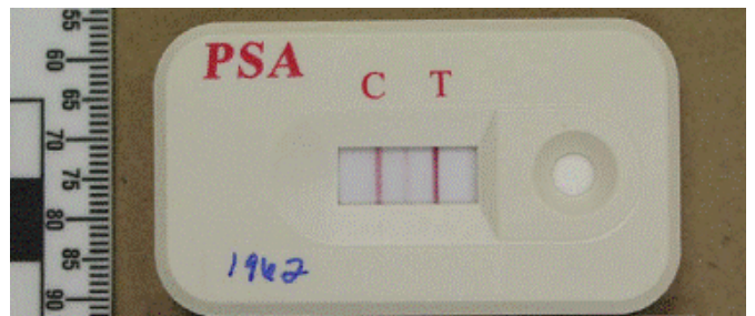
FIG. 4—Seratec® PSA membrane card after the addition of an extract from a seminal stain deposited on cloth and stored at room temperature since 1962. The first line (from the left) is a control line that must develop to ensure the test is working properly. The second line is an internal standard that is adjusted to the color intensity of a PSA stain of 4 ng/mL concentration. The third line is the test line and is quite obviously positive with a concentration of PSA in excess of 4 ng/mL.
